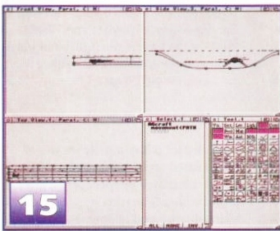
15 Enter the new level and select the menu Create/Controls/b-spline knot. Define a curve, starting from the craft by setting knot points, that goes part way down the track and then doubles back up to the start.
